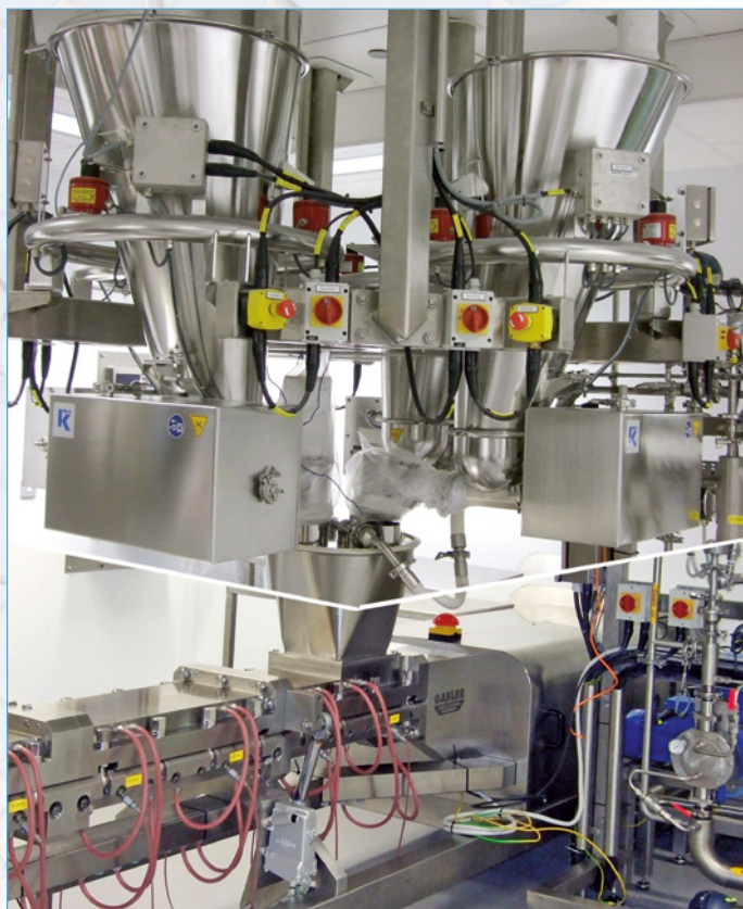
A group of Coperion K-Tron Pharma Feeders feeding directly into an extruder inlet
